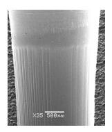
拉痕: 一种于拉拔方向一致的沟痕。Stretched marks: a groove marks in accordance with drawing direction
